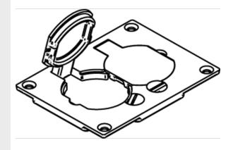
Brass duplex cover plate, 3.156" x 4.182" [80.2mm x 106.2mm]. Flip lids can also be used with 106 type frames for communications. NOTE: Brass covers and flanges are not interchangeable with aluminum or nonmetallic covers and flanges. Nonmetallic covers are interchangeable with aluminum flanges.
