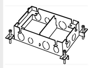
The 880M2 Omnibox Floor Box Series provides an excellent activation solution for applications where single service is required in open space areas. The 880M2 Floor Box is offered in a stamped steel construction, designed to be installed in above grade concrete floor applications and to meet a wide range of market requirements.
