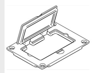
Brass GFI cover plate, 3.156" x 4.182" [80.2mm x 106.2mm]. May be used with Wiremold CM Series adapters and Ortronics Connectivity Systems in conjunction with 817B, 827B, and 837B Flanges. features & benefits
