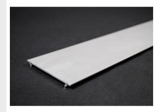
Satin anodized finish. Nominal wall thickness of .078" [1.99mm]. Packed eight 5' [1.50m] lengths per carton. ALAC-5 is compatable with ALA3800 and ALA4800 Series Raceways.
