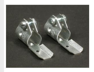
Connects 14/2, 14/3, 12/2, and 12/3 "MC" and armored cable to Wiremold fittings. A short piece of 500 or 700 Series Raceway (1 5/8" [141mm] min.) must be used between connector and Wiremold fittings. Not for use with 1/2" [12.7mm] flex conduit.
