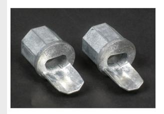
Interior threaded female connector for connecting raceway to conduit. When used with 700 Series Raceway, break out crescent twistout in connector. 5782 has 1/2" trade size conduit opening and 5782A has 3/4" trade size conduit opening.
