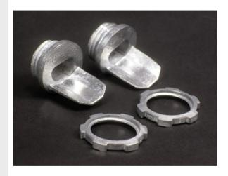
Male connector for connecting raceway to conduit boxes or panel boxes that have KOs for conduit. Can also be used with conduit type fittings. When used with 700 Series Raceway, break out crescent twistout in connector. 5781 has 1/2" trade size conduit opening and 5781A has 3/4" trade size conduit opening.
