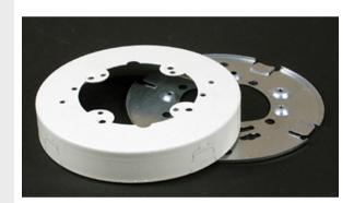
Mounts onto 3 1/4" or 4" [83mm or 102mm] conduit boxex, or other recessed outlets. Cover accepts devices with mounting screw centers of 2 3/4", 3 1/2", or 4 1/16" [70mm, 89mm, or 103mm]. Can be used with 5736 Blank Cover as a pull or junction box. Outside diameter 5 1/2" [140mm].
