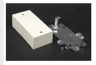
Can be used as tee, cross, pull box, junciton box, or blank box. Cover has 1/2" trade size KO and twistouts for 500 and 700 Series Raceway on each end and sides. Twistouts on ends of box permit running raceway close to interior trim. Base has 1/2" trade size KOs.
