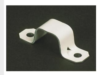
Converts to one-hole by breaking off at score. Lanced tab holds strap in place while fastening to surface. NOTE: Use #8 panhead screws.
