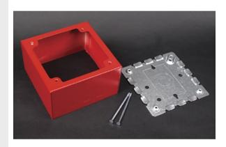
For surface mounting of alarm devices and safety signals designed to fit into 4" [102mm] square back boxes. R5753 has red finish. Cover is 2 3/4" [70mm] deep and has three twistouts for raceways on each side. Base has 1/2" and 1" concentric and single-gang box KOs. Accepts NEMA double-gang standard faceplates.
