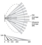
Coverages shown are maximum and represent half-step walking motion. Under ideal conditions with no barriers or obstacles, coverage for half-step walking motion can reach up to 2000 ft $^2$ , while coverage for typical desktop activity can reach up to 1000 ft $^2$ .
