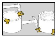
attachment of pipe sleeves to wall and floor forms for concrete pouring.
