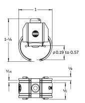
Steel connector for attachment of non-metallic sheathed cables to enclosures and junction boxes. For residential and commercial applications.
