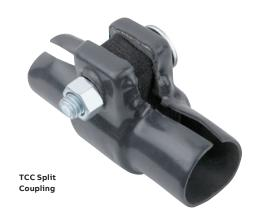
Split couplings serve as speed unions for costeffective joining of two separate lengths of threaded conduit. Like other Ocal® fittings, they're double coated in urethane and PVC to safeguard your entire conduit system against corrosion.
