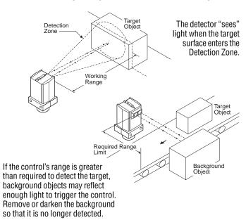
then remove or darken the background. If that is not possible, move the sensor farther away from the background, making sure it will still detect the target. If the background has a glossy or shiny surface, angle the sensor in relation to the background to eliminate direct reflection.
