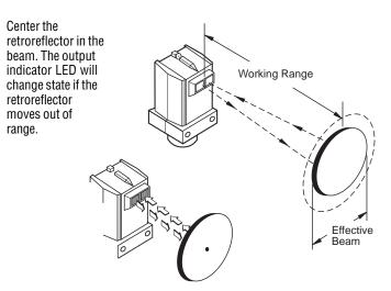
Polarized models "see" only light rotated 90°. Polarized light is rotated 90° by the retroreflector.
