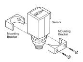
into the sensor. Use two 0.203 inch diameter holes drilled 1.18 inches apart. The ball swivel feature allows a 10° tilt from vertical, and a 360° rotation to aid alignment.
