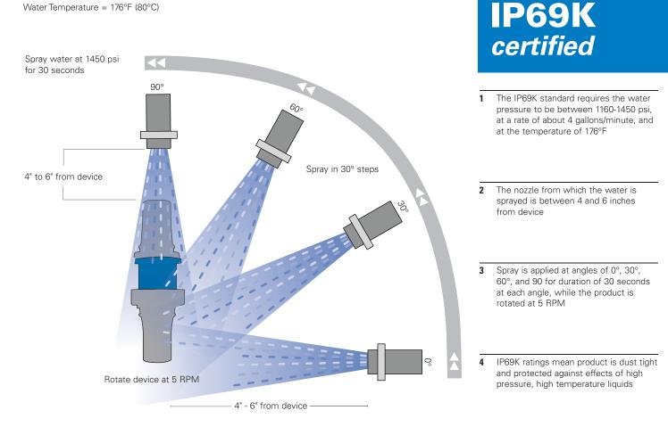
After testing, water must not be present inside the device
