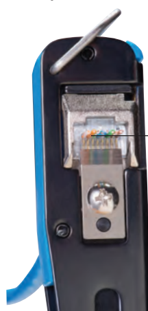
568A & 568B wiring scheme marked on tool
