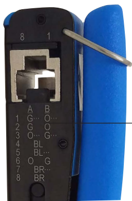
568A & 568B wiring scheme marked on tool
