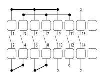
Custom rotary switch options include engraved faceplates, master key systems, and contact behavior configurations (illustrated left).
