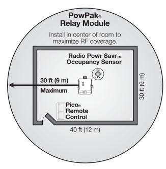
All Wireless Transmitters must be installed within 30 ft (9 m) of the PowPak<sub>®</sub> Relay Module.
