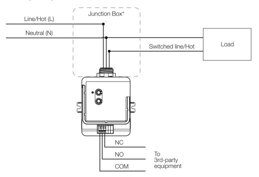
\* NOTE: Some applications (in U.S.A.) require the PowPak® module to be installed inside an additional junction box. For information about how to perform this installation, please visit www.lutron.com, Application Note #423 (P/N 048423). Please consult all local and national electric codes for proper installation methods.
