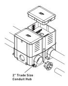
Box comes complete with reusable mudcap, insert spacer, conduit plugs and reducers. Reducers provided for reduction to 1 1/2", 1 1/4", 1", 3/4", and 1/2" [25mm, 19.1mm, and 12.7mm] conduit. Minimum concrete depth is 4" [102mm] and maximum concrete depth is 6" [152mm]. Minimum capacity is 50 cu. in. [819ml] and maximum capacity is 100 cu. in. [1693ml]. Box dimensions are 4 1/8" W x 5 1/2" L x 6" H [105mm W x 140mm L x 152mm H].
