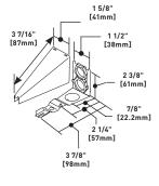
Eliminates need to offset raceway when connecting to surface type panel boxes. Adjustment from surface to center of bushings is 5/8" [15.9mm] minimum to 1 3/8" [35mm] maximum. When used as adjustable offset connector, break out metal between the two holes. When used with 700 Series Raceway, break out crescent twistout in cover. 1/2" trade size chase nipple and locknut furnished.
