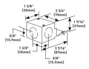
Connects 3000 Series Raceway to 1/2" trade size conduit and armored cable connectors. 1/2" trade size KOs on end and each side of fitting. Can be connected to conduit boxes by using 1/2" chase nipple.
