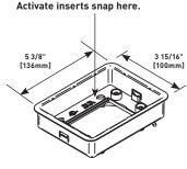
Comes with fiber storage loop. Also includes brass inserts for flange connection and green ground wire for ground connection. Wiremold CM Series Open System adapters that snap directly into the adjusting ring without the need for an adapter. Also includes mounting screws to attach flange to box body.
