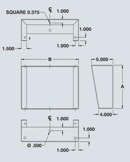
The 885 MF - Floor mounting feet are made from 14 GA steel, predrilled for fixation to the floor and to the bottom of the 5412 and 5500 series enclosures. Kits come complete with all necessary hardware. Mounting feet are finished with heat fused polyester powder, electrostatically applied on a phosphatized base. Finish is ANSI/ASA 61 gray.
