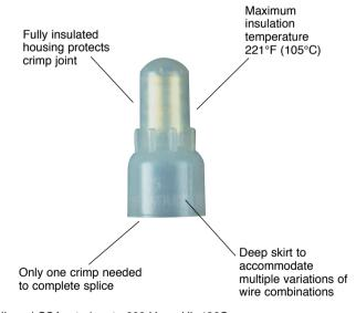
UL and CSA rated up to 600 V per UL 486C. Metric versions available. Flammability - UL 94 HB.
