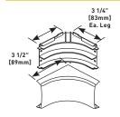
A 90° internal corner with integral dividers provide 2" [51mm] cable bend radius for UTP and fiber optic installations. Also available in white (2317DF0-WH).
