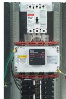
The SPD Series is also available as an integrated unit interfaced via a circuit breaker unit interfaced via a circuit breaker resident in the electrical assembly. This installation keeps connected lead lengths short while providing a means of disconnecting power to the unit quickly and easily.
