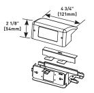
Accepts two Extron® Electronics MAAP single space modules.
