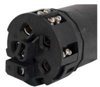
Tapered wiring pockets to ease insertion of stranded wire; deep pockets with clear markings keep bare conductors isolated
