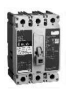
The Non-padlockable Handle Block secures the circuit breaker handle in either the ON or OFF position. (Trip-free operation allows the circuit breaker to trip when the handle block holds the circuit breaker handle in the ON position.) The device is positioned over the circuit breaker handle and secured by a setscrew to deter accidental operation of the circuit breaker handle. CSA and UL listed. (Field installation only).
