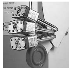
Triple Padlocking Capability
