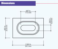
The barrier strip clamp is used to mount barrier strips to ExpressTray™ profiles. Available in electro-galvanized steel, hot-dipped galvanized steel and stainless steel (304 and 316).
