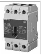
The new NGG Circuit Breaker is a compact, industrial design with true value-added features such as Global Ratings (UL/CSA/IEC/CE/NOM), flexible DIN or base mounting without the need for adapters and UL Listed for field install-able accessories. This NGG125 has a 25KAIC interrupting rating at 480VAC and features a Quick Make/Quick Break Trip-free Mechanism. All this in a 3.0W x 5.4H x 2.8D package. Please consult your sales office for availability.
