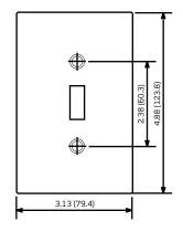
Note: Add 1.81" (46.0mm) for each additional gang. Midway wallplates can be mounted onto larger-volume outlet boxes and/or used to hide wall irregularities. Midway wallplates are a full 0.375" taller and wider than standard size wallplates.
