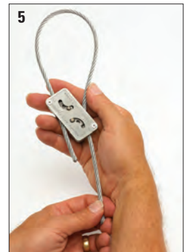
5 To adjust, remove tension and pull wire rope slightly to disengage teeth, slide adjustment pin in direction shown by arrow to release wire rope.
