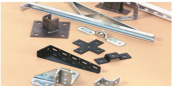
This section offers a full selection of fittings and accessories to complete our strut system. Fittings are made from hot rolled, pickled and oiled plate or strip steel in accordance with ASTM A1018 33,000 PSI min. yield, unless noted.
