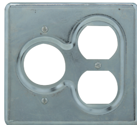
For round flush receptacles (hole diameter 1 13/32 ""); duplex convenience receptacles, standard and 2-wire, 3-pole grounding (hole diameter 1 11/32 "")
