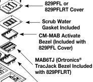
MAB3S2 Bezel (Ortronics® Series II Bezel Included with 829PFLRT) Fiber Optic Installation (Activate Only).
