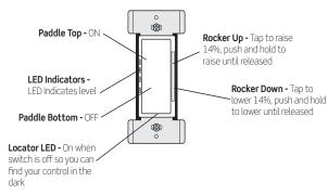
\*Default configuration shown. Buttons can be programmed with any function, ex: scene, raise/lower, toggle, etc.
