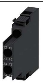
LATERAL AUX.SWITCH BLOCK,SIDE, 2NO, CURR.PATH: 1NO, 1NO, FOR MOTOR CONTACTORS, SZ S00, SCREW TERMINAL R: 23/24, 33/34 L :43/44, 53/54
