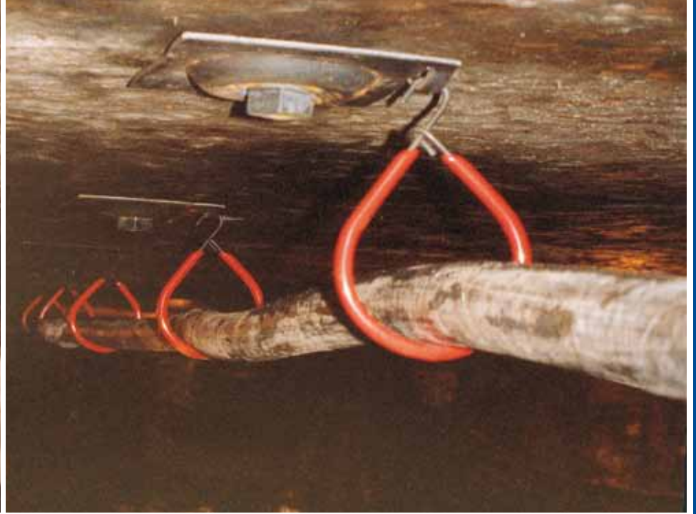
All hanger carrying surfaces are fully insulated with a tough, high dielectric grade, flame retardant plastisol coating.
