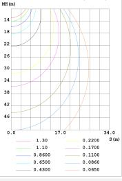
CO PLANE ISOLUX DIAGRAM (UNIT:1x)
