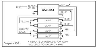
Note: When retrofitting with an instant start system to replace a rapid start system, some modifications to the socket wiring are necessary for optimal performance. This requires the two lamp pins to be shunted as close to the socket as possible. Do this by either installing shunted sockets or installing a jumper wire to tie the two lamp pins together in each socket. Failure to shunt the pins together will cause the lamps to fail prematurely.
