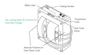
Philips Advance HID Core & Coil ballasts are date stamped on either the top surface or the side surface of the ballast core. The four-digit number represents the week and year of manufacture. The first two numbers indicate the week and the last two indicate the year the ballast was manufactured. The example shows a ballast manufactured during the 36th week of 1989. The three letters are a factory code.
