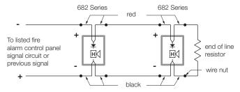
Polarity of signal circuit shown in supervisory state. On alarm the polarity reverses.
