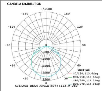
Efficiency Total: 100% Lumen Rating: 6541 Efficacy Total: 85 lm/W Input Wattage: 77W
