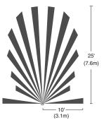
The CN and CW have a coverage range of 180 degrees and a maximum coverage area of 300 ft<sup>2</sup>. To maintain its coverage capacity and optimally detect motion, the sensor must have a clear and unobstructed view of occupants.
