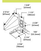
Eliminates need to offset raceway when connecting to surface type panel boxes. Adjustment from surface to center of bushings is 5/8" [15.9mm] minimum to 1 3/8" [35mm] maximum. When used as adjustable offset connector, break out metal between the two holes. When used with 700 Series Raceway, break out crescent twistout in cover. 1/2" trade size chase nipple and locknut furnished.
