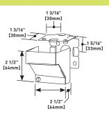
For feeding raceway from ceiling or floor. Allows for ample splice room. Base has 1/2" trade size KO.
