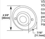
Blank Cover - Use with V5735, V5737, V5737A, V5738, V5738A, V5739, or V5739A, or V2135 converting them to pull or junction boxes and for hanging lightweight pendant fixtures having 1/2" [12.7mm] pipe stems, etc. Has 1/2" trade size KO.
