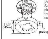
Fan Box/Solid Base - UL approved fixture box for ceiling fans. Cover accepts fan brackets with 3.2" [82mm] mounting centers. Supports up to 50 lbs. Base has six mounting holes and four 1/2" trade size KOs. #10 mounting screws provided.
