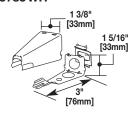
Combination Connector - For connecting raceway, without offsetting, to any 3 1/4" [83mm] or 4" [102mm] outlet box mounted on the surface with a KO for 1/2" [12.7mm] conduit. The base end and bottom has two 1/2" trade size KOs. Break off cover extension to use with 700 Series. Spring steel bushing included for end connection to box, eliminating conduit nipple and locknut.
